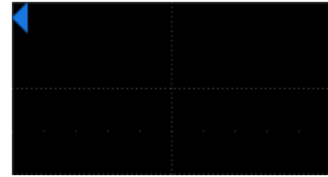
Horizontal 0 position (out of screen) Indicator
